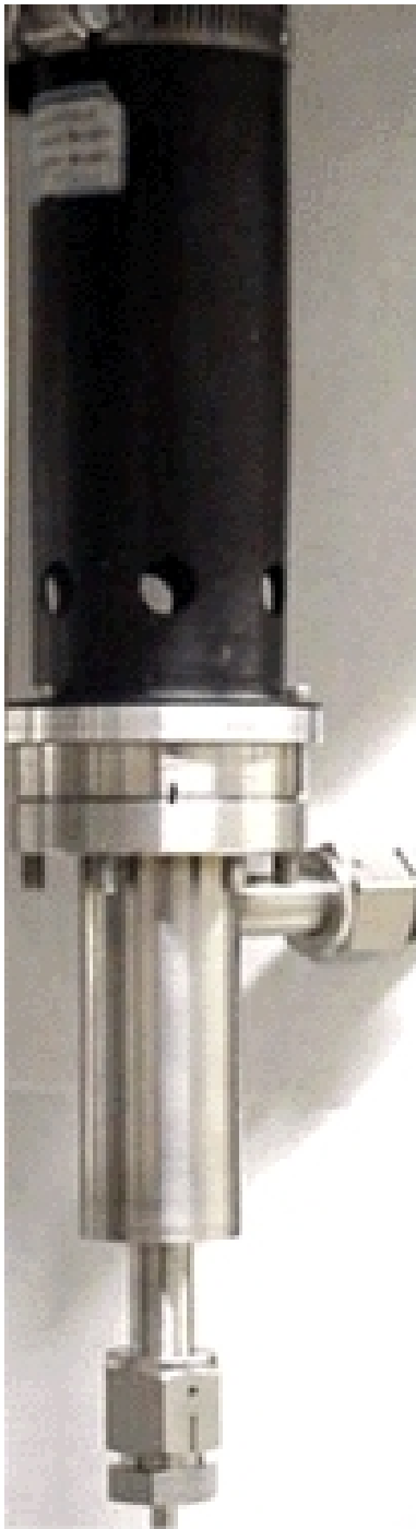
Tritium Signal Processor with 10cc ion chamber
